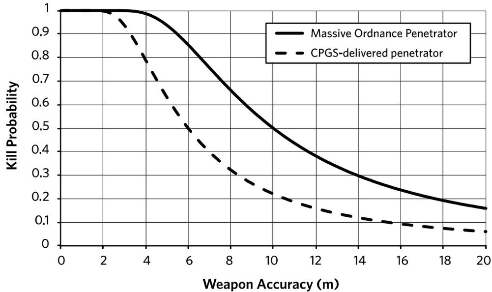
**FIGURE 1: Graph of the Kill Probability of the GBU-57 (Massive Ordnance Penetrator) and a CPGS-Delivered Penetrator Used Against an SS-18 Silo as a Function of Weapon Accuracy.** Technically, weapon accuracy is given by the circular error probable. For details of the calculation see James M. Acton, “Hypersonic Boost-Glide Weapons,” (forthcoming).
